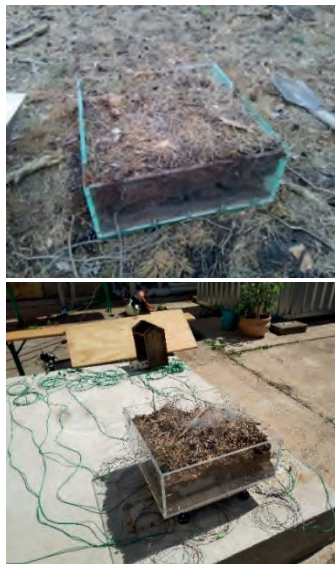
Abbildung 2: Small scale fire tests, soil specimen from forest near Calvörde (Saxony-Anhalt)
